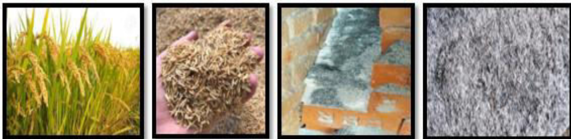
Fig 1: Production of Rice Husk Ash
